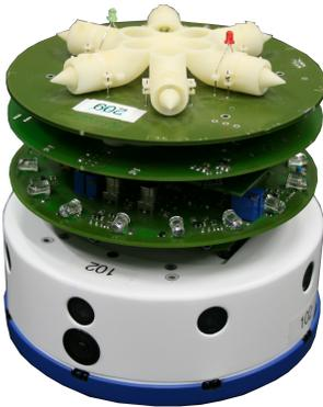
Fig. 3. The Khepera IV robot with custom relative position, odor and wind measurement extension boards.
